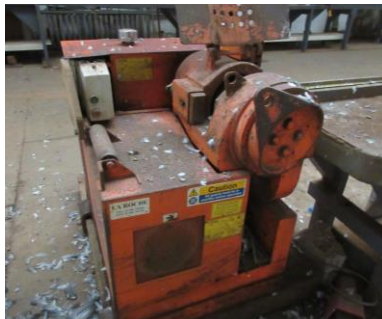
La Roche bar bending & cutting machine (Zoff)
