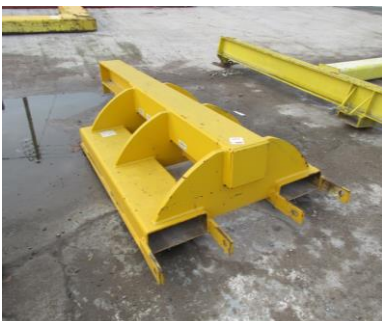
Contract forklift attachment lifting jib, 18,000kg (2023)
