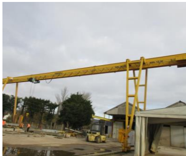
Pelloby 12.5 ton 50m span rail mounted portal yard crane (2019)
