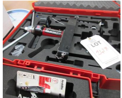
Hydrajaws fixing tester, model 2050
