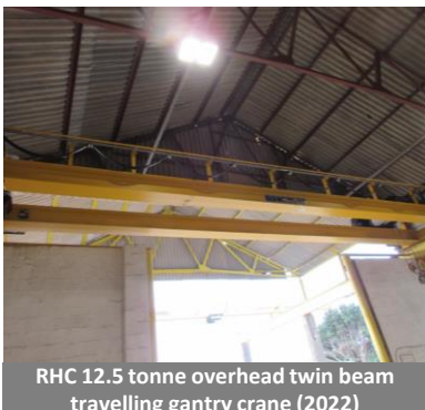
Demag 12.5T overhead twin beam travelling gantry crane
