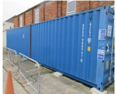
Export type shipping container, 8' x 40', fitted out as drying room
