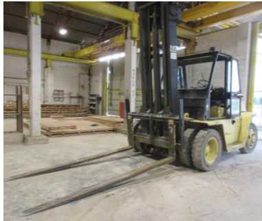
CAT V180B diesel dual mast forklift truck
